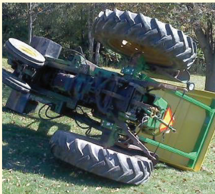
Mr. James Daum's tractor rests on its side after a rollover. The newly-installed roll bar protected Mr. Daum during the incident. (Photo courtesy of Mr. James Daum.)
