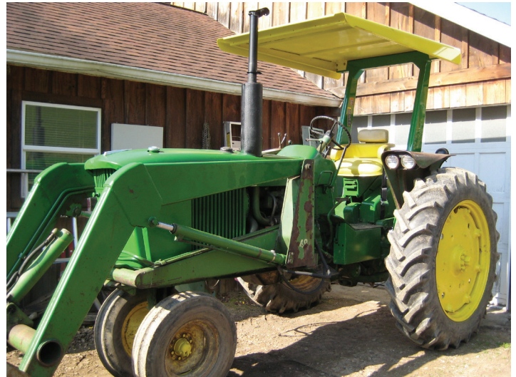
After roll bar installation. (Photo courtesy of Mr. James Daum.)
